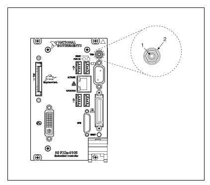
Figure 3-7. TRG Connector Location and Pinout
